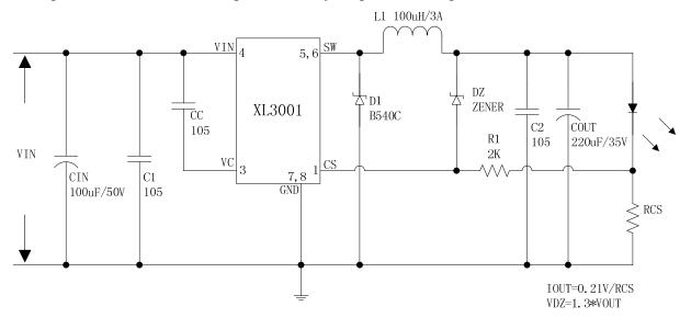
Figure 19. XL3001 System Parameters Test Circuit (LED OVP)
