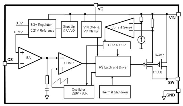
Figure 3. Function Block Diagram of XL3001
