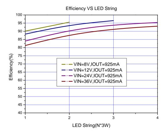
Figure 17. XL3001 System Efficiency Curve
