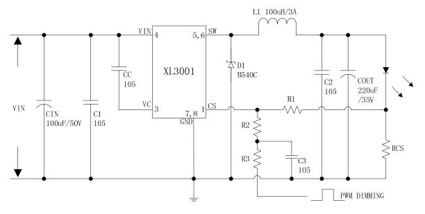
Figure 18. XL3001 System Parameters Test Circuit (PWM DIMMING)
