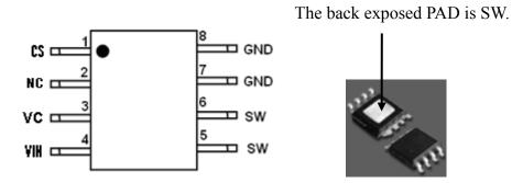
Figure 2. Pin Configuration of XL3001 (Top View)
