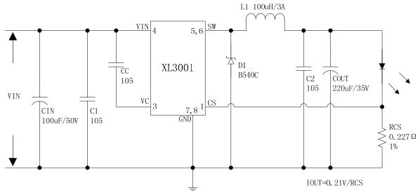
Figure 16. XL3001 System Parameters Test Circuit (VIN=8V~40V, IOUT=925mA)
