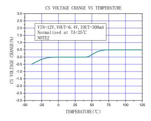
**Note2:** Internal temperature compensation circuitry is provided to compensation the PCB and external line loss in system application. When the junction temperature or the output power rise, the CS voltage will be compensated. This function is provided to compensation the PCB and external line loss in system application.
