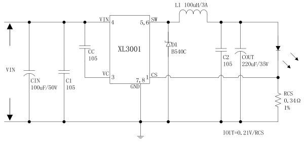
Figure 14. XL3001 System Parameters Test Circuit (VIN=8V~40V, IOUT=615mA)
