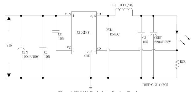
Figure 4. XL3001 Typical Application Circuit
