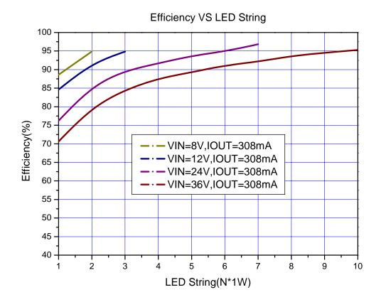
Figure 13. XL3001 System Efficiency Curve
