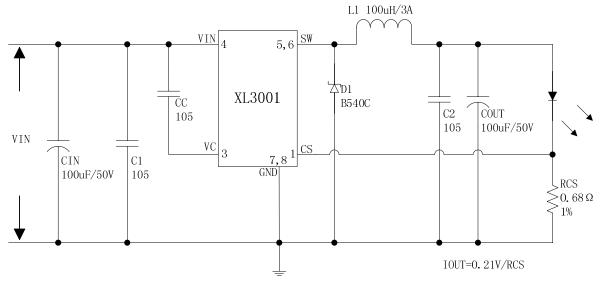
Figure 12. XL3001 System Parameters Test Circuit (VIN=8V~40V, IOUT=308mA)
