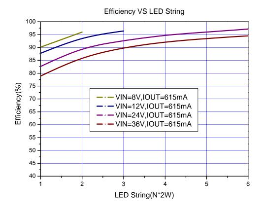
Figure 15. XL3001 System Efficiency Curve
